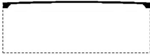
Fig. 13 Resulting topology for the minimum compliance with thermal load problem formulation
