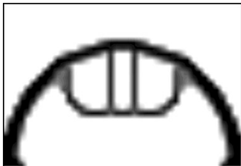
Fig. 17 Pressurized arch: solution obtained with continuation method ( m = 1449.42 )
