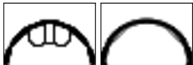
(a) Compliance minimization from stress solution ( C = 6185.43 )
