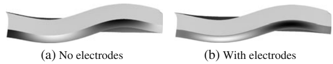
Fig. 4 Electric potential induced by harmonic mechanical displacement to the system (Fig. 1). If there were no electrodes as in (a) local compression and expansion results in electric potential of opposite sign within \Omega_p but also at the surfaces \Gamma_{\text{gnd}} and \Gamma_{\text{hot}} . With electrodes (b), the electric potential averages both on \Gamma_{\text{gnd}} and \Gamma_{\text{hot}} to zero
