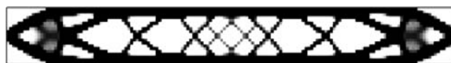
Fig. 6 Single-material topology design (50% volume fraction) obtained by maximizing the first eigenfrequency of the simply supported beam-like structure in Fig. 2a by the using the mean eigenvalue approach. The design may be compared with the optimum design in Fig. 3a
