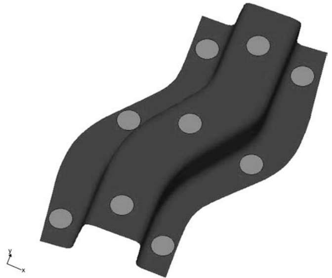
Fig. 4 Points used to measure the distance between the desired geometry and the simulation result in the SRAIL test case
