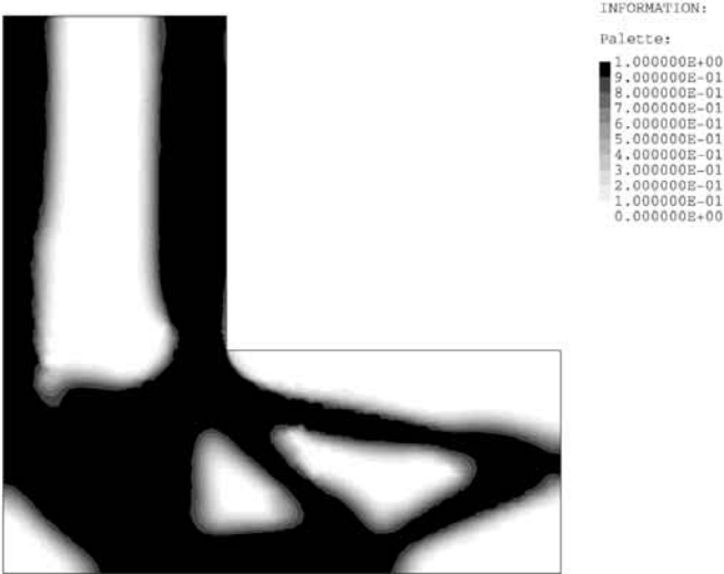
Fig. 13 Minimum mass approach: final density for \epsilon = 0.05
