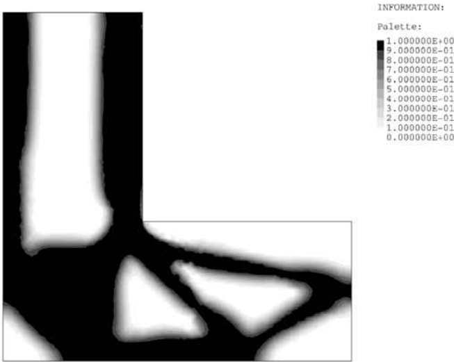
Fig. 12 Minimum mass approach: final density for \epsilon = 0.1
