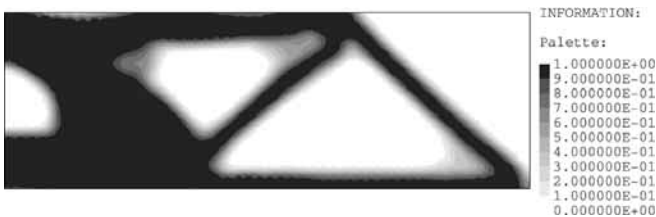
Fig. 19 Minimum mass approach: final density
