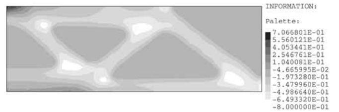
Fig. 22 Minimum compliance approach: \epsilon -relaxed failure function
