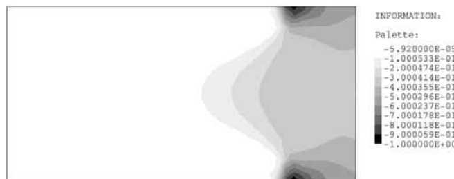
Fig. 5 Traction load case: \epsilon -relaxed failure function
