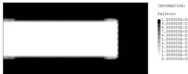
Fig. 6 Bending load case: final density
