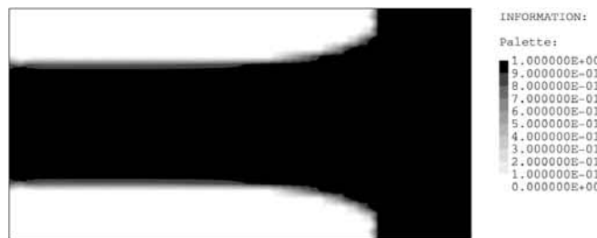
Fig. 4 Traction load case: final density
