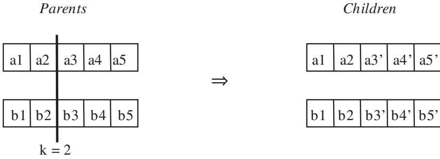
Fig. 2 Description of the cross-over operator a'_i = b'_i = (a_i + b_i)/2 for i > k
