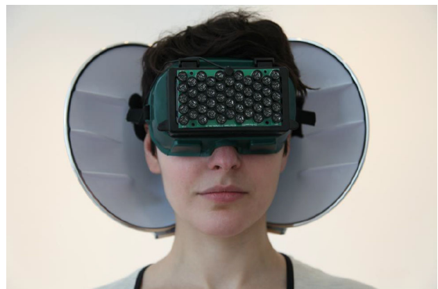
Fig. 3 First iteration of the Echolocation Headphones with augmented false auricles
