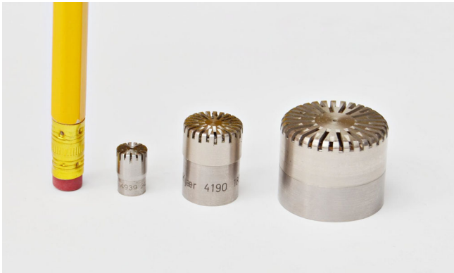
Fig. 1. Microphone capsules (from right to left ): Brüel&Kjær 4145 (1" diameter), 4190 (1/2" diameter), and 4939 (1/4" diameter). A common pencil is included for size comparison.
