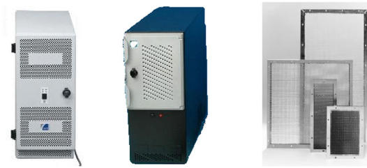
Fig. 27. Examples of electromagnetic shielding with perforations and meshes. The two computers meet the strict NSTISSAM TEMPEST/1-92 Level I requirements for electromagnetic side channel emanations, yet have ample ventilation holes (catalog photos, left Advanced Programs, Inc., model DWT-105; middle EMCON Emanation Control Limited Core 2 Quad workstation). On the right are shielded honeycomb air vents (Parker Chomerics CHO-CELL panels of several sizes, “especially designed for high-frequency environments and to meet TEMPEST specifications”).
