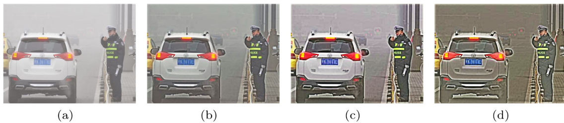
Fig. 5 Ablation study on the patch size in dark channel loss. a is the hazy image. The patch size in b is 4 \times 4 , in c is 8 \times 8 , and in d is 16 \times 16
