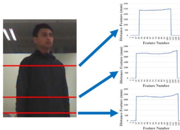
Fig. 6 Curves as the function of the distance of the projected horizontal lines on the human upper body area at \alpha = -30^\circ
