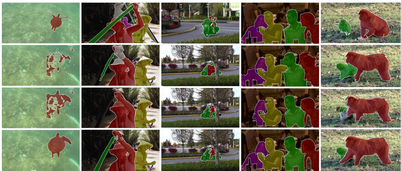
Fig. 10 Visualization results on the DAVIS Test-Challenge dataset. From top to bottom: the first video frame with the ground-truth label followed by results of our proposed methods in pre-view segmentation [26], contextual segmentation [59], and guided segmentation [58]. The
