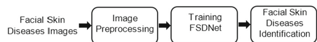
Fig. 1 Block diagram of the suggested method. The images are first collected and labeled. They go through some preprocessing techniques such as resizing to fit the network, data augmentation to increase the size of the dataset, and then feeding to the network to be trained to finally identify the appropriate class
