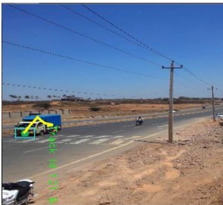
Fig. 7 Results of vehicle detection and speed estimation of video sequence 5
