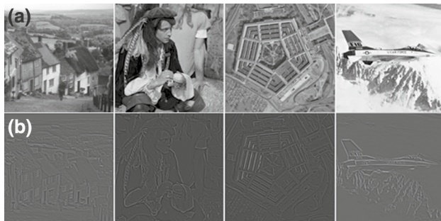
Fig. 1 Examples of NSS features extracted from images. a some natural images from the standard test dataset; b the contours according to a (extraction with second atom by using PCA method)
