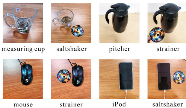
Fig. 1 Examples of real-world adversarial patch attacks against VGG 16. We can observe that each object is misclassified when the adversarial sticker is placed beside it
