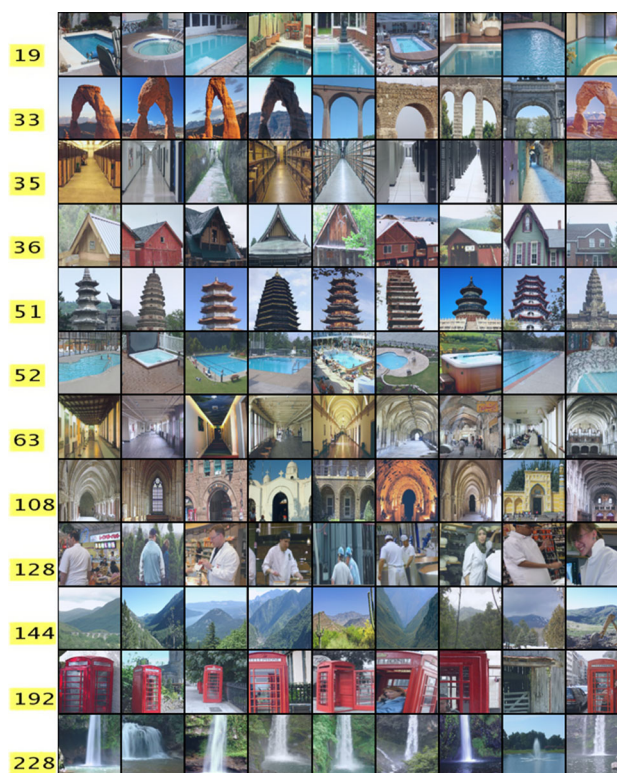
Fig. 1 Visualization of the maximally activated image regions for few filters (19, 33, ..., 228) of CONV5 layer of Places365-AlexNet [24] on images of SUN397 scene dataset [45]. Activated regions on same row correspond to a concept
