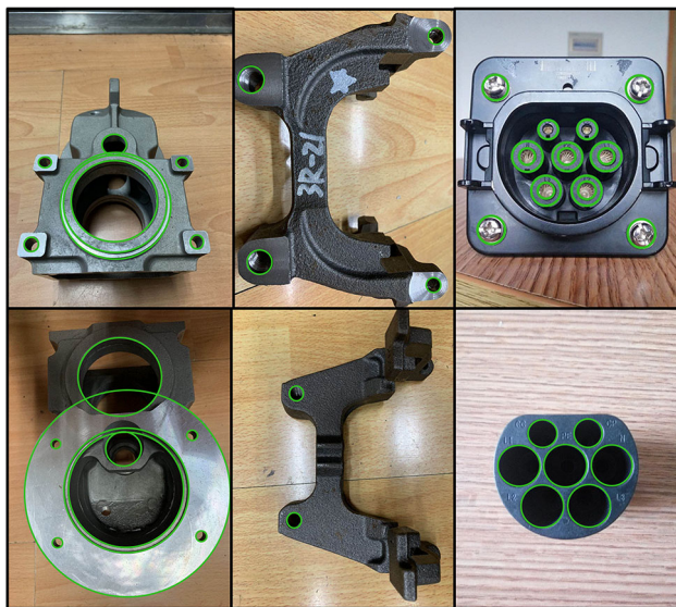
Fig. 28 Application examples of ellipse detection for mechanical parts
