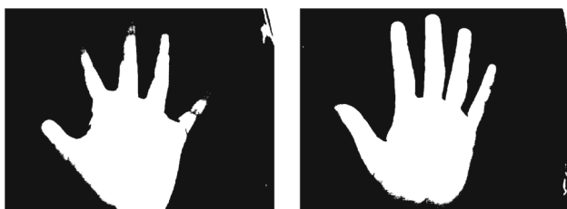
Fig. 11 Two binary images showing the segmentation failure cases in our database
