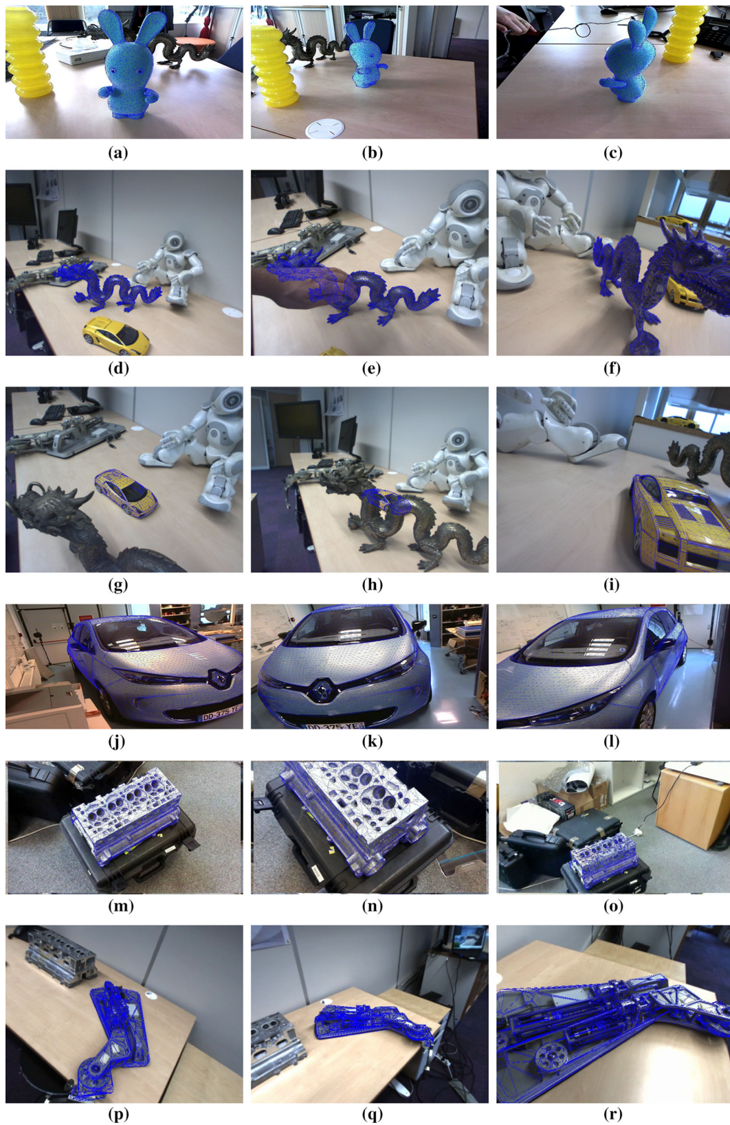
Fig. 26 Accurate localization results on a Raving Rabbid, a dragon, a sport car, a real-sized car, a car cylinder head, and an orthosis with our phDEC-SLAM. Results are similar with rDEC-SLAM and rhDEC-
