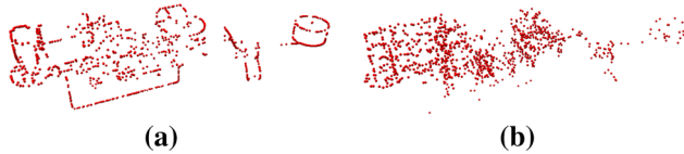
Fig. 12 Set of edgelets extracted by using our sampling method on the left and with a random sampling solution on the right
