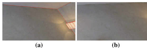
Fig. 23 Our DEC-SLAM is not able to estimate camera poses when any model information or environment keypoints are available to constrain our method. Without depth information, our solution fails when the camera is looking at planar textureless regions. a, b Frames from the ICL-NUIM kt0 sequence [9]. The tracking is lost when only walls are visible
