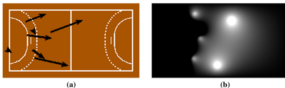
Fig. 3 Generating a motion-information image using frame differencing. a Team players movements. b The motion-information image
