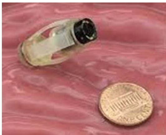
Fig. 8 Robotic magnetically actuated soft capsule endoscopes (MASCE) [34,35]
