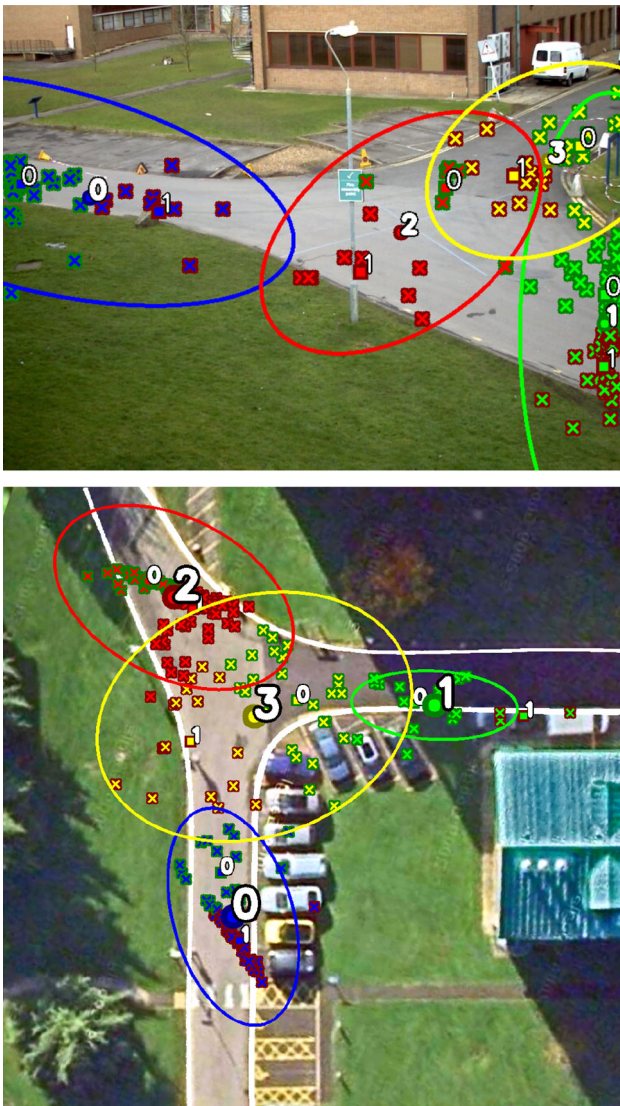
Fig. 12 Goal clustering. Top : Results in image plane. Bottom : Clustering in world plane. The circles depict the centroids computed by the clustering algorithm, the crosses are the key points and the ellipses show the covariance of each cluster. The color of each element is the one of the closest centroid
