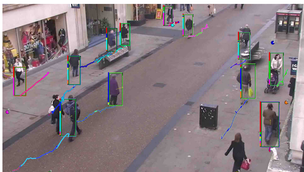
Fig. 11 Tracking on the TownCentre dataset. The ground-level lines depict the target trajectory, where the color indicates the most probable goal at each instant
