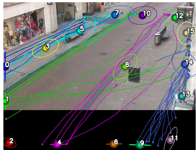
Fig. 3 Clusters obtained with training trajectories from the Town Centre video sequence [6]. The circles and the crosses depict the starting and ending points of each sub-trajectory, respectively. The colors are related to each of the six clusters, and the sub-trajectories take the colors corresponding to their associated goals
