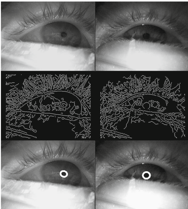
Fig. 12 Successfully found pupils by the ElSe algorithm in eye images from Data set XXI
