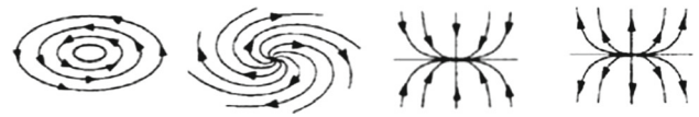
Fig. 2 Critical points of typical flow fields : vortex, whirl, attractive and repulsive point
