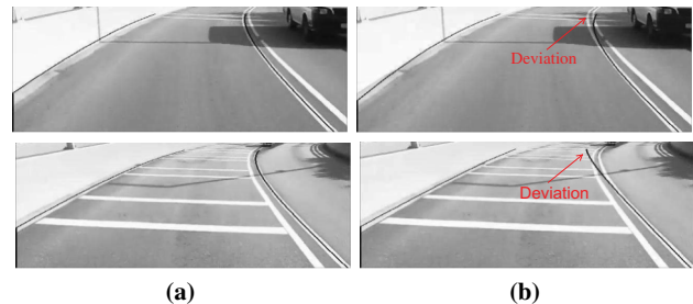
Fig. 18 Comparison of fitting results between modified (column a) and conventional (column b) RANSAC
