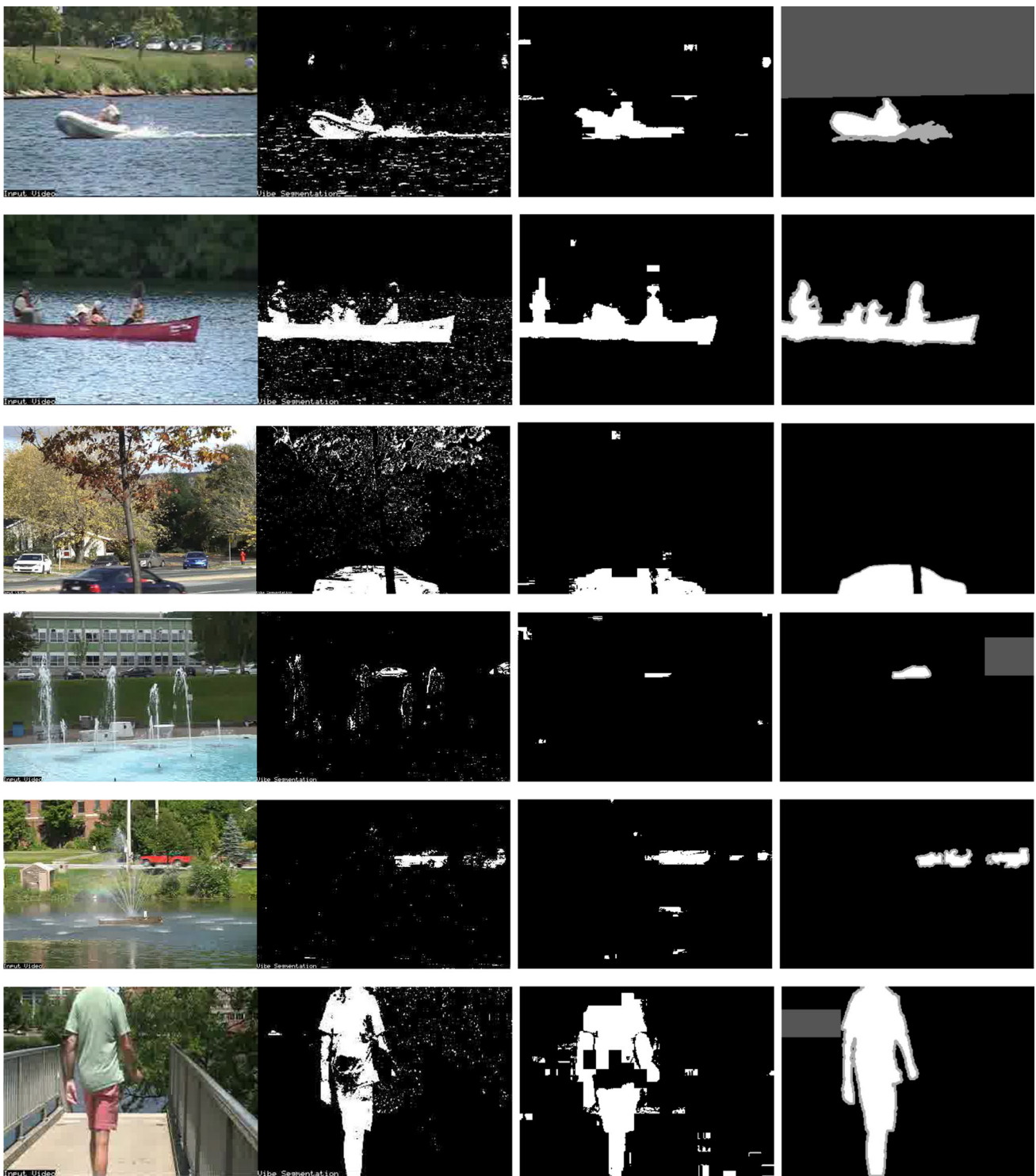
Fig. 15 Background subtraction results from the change detection dataset category of dynamic background—original image frames and results obtained by VIBE ( first column ), results obtained by TSBS ( second column ), ground truths ( last column )
