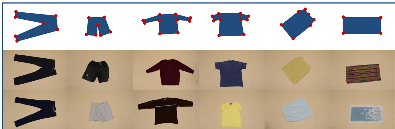
Fig. 3 Top synthetic templates of unfolded garments belonging to six different garment types. Landmark points used for producing the SMPs are denoted by red dots on the templates' contours. Bottom images of
