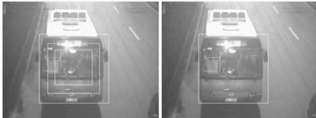
Fig. 7 The containment relations for the bounding boxes and the final result from deleting the smaller ones
