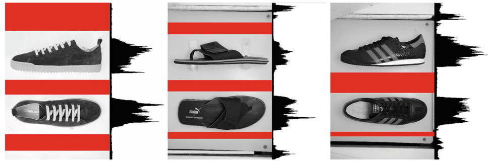
Fig. 2 Vertical gradient projection histograms are used to highlight slices that probably belong to the background (highlighted in red)
