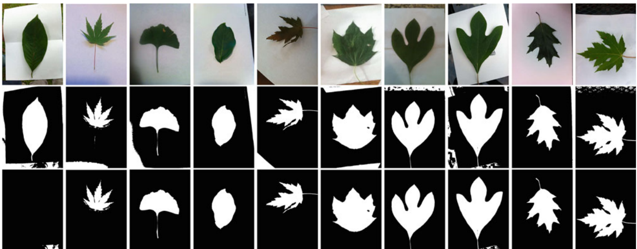
Fig. 12 Segmentation results on the User dataset illustrating the effects of post-processing. From top to bottom original image, result of EM, and result of EM P (EM with post-processing). The images are ordered by the overlap ratio between the two segmentations, so that the left-most has the most dissimilar segmentations, with the similarity increasing as we move right . In order to better illustrate the range of differences, every eighth image is shown. Note the post-processing procedure was in error on the left-most image, though in all the other images it improved the segmentations. The post-processing error on the leftmost
