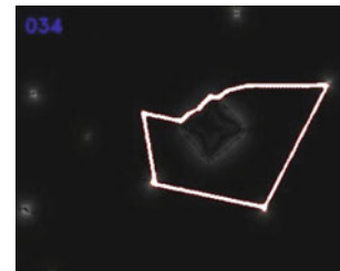
Fig. 6 Segmentation failed because of noisy edge image
