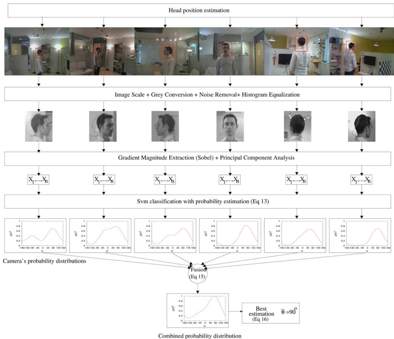
Fig. 2 General scheme of the proposed solution. Head images are extracted and then preprocessed. The n first principal components are the input for an SVM classifier. A probability distribution of the head angles is obtained for each camera and then fused to obtain the best estimation
