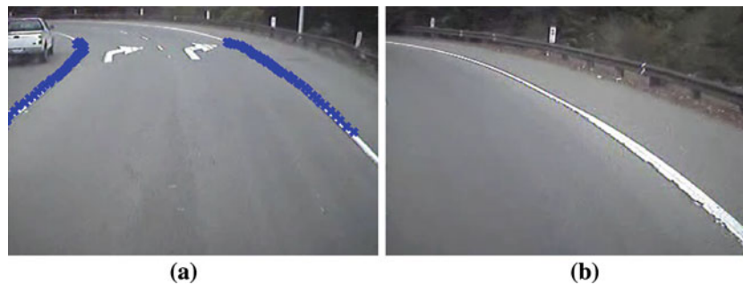
Fig. 16 Method 2 in large curvature situation (Frames are from Zu [14]). a Large curvature with two lane boundaries available, Method 2 works, as well as will Methods 1 and 3 . b Large curvature with only
