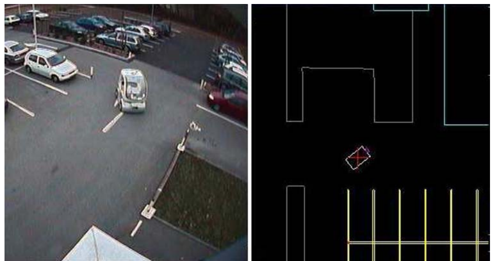
Fig. 15 The ParkView platform: left camera view of the Cycab experimental car moving in the parking lot of the laboratory; right the Cycab as detected on the tracking system
