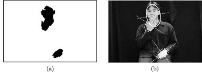
Fig. 2 a Occlusion of the face and the right hand is shown as one merged object as a result of skin colour detection. b Segmentation algorithm separates the hand and the face to extract their corresponding geometric features
