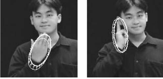
Fig. 3 A close-up view of the snake initialisation shows the previous snake in thin line, the optical flow calculated for each snake point, and the initialised snake for the current frame in thick line
