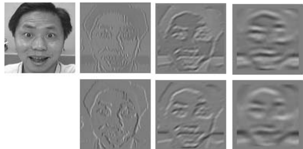
Fig. 4. Convolution results of one image with three Gabor kernels
