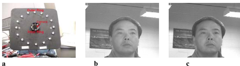
Fig. 1. a IR camera with active IR illuminator. b Bright pupils in an even field image. c Dark pupils in an odd field image
