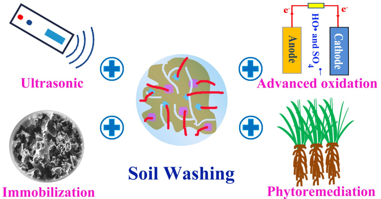
Fig. 3 Main remediation technologies combined with soil washing
