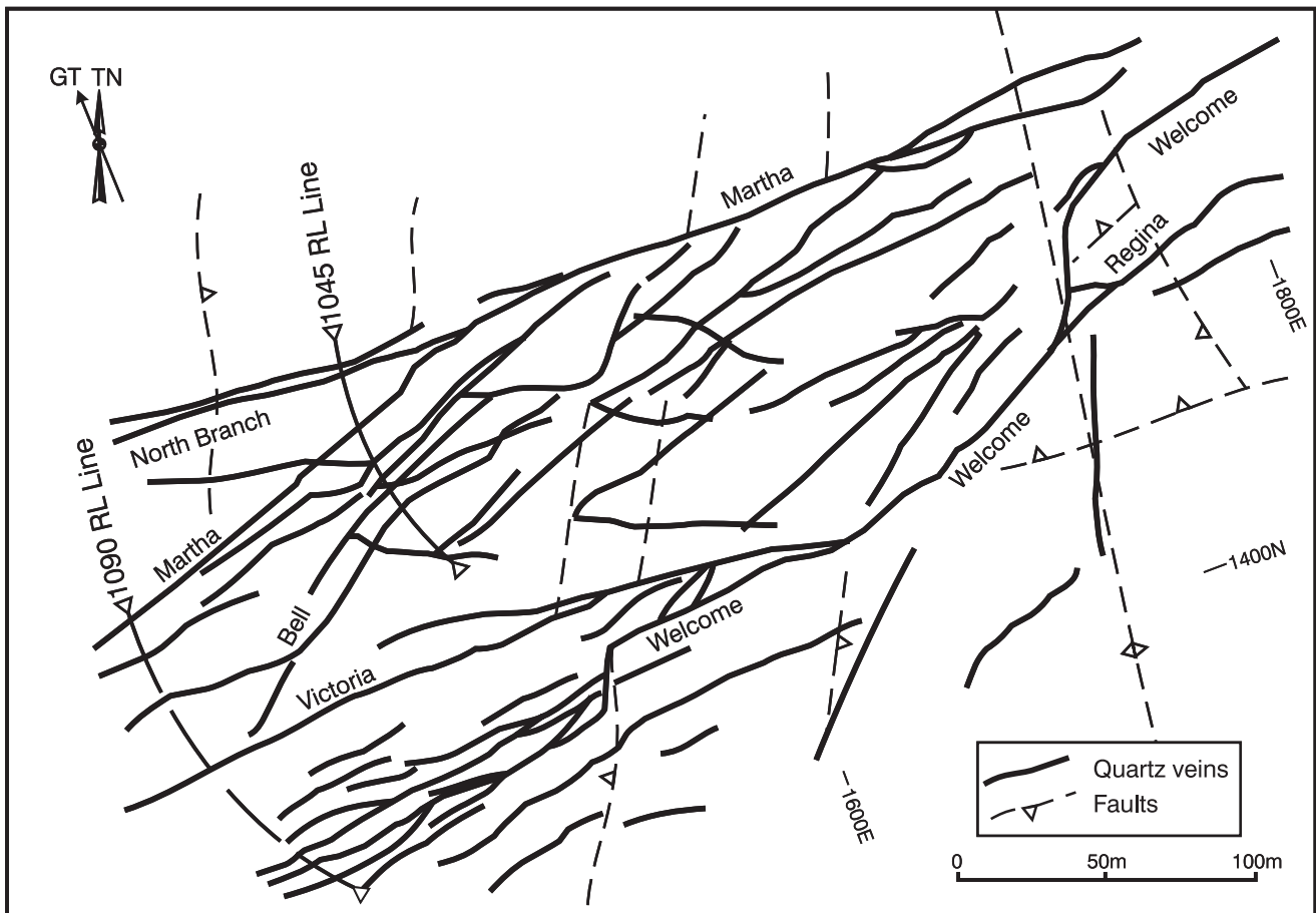
Fig. 5 Plan of major quartz veins (veins thicker than 0.1 m) in the Martha Hill open pit at 1100RL (after Cargill 1994), with location of line samples at 1090RL and 1045RL. Thickness of veins not shown
