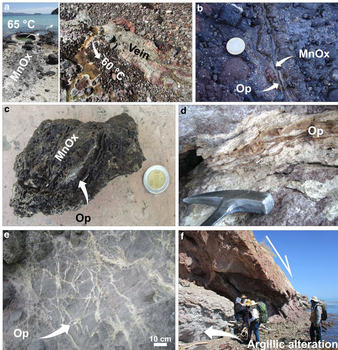
Fig. 2 Field photos of the main coastal hot spring sites and mineralization styles of the Bahia Concepcion. a Coastal hot springs at Mapachitos and Posada Concepcion, arrows indicate direction of discharge. b Symmetrical banded opal and Mn oxide veinlet. c Hand specimen of a
