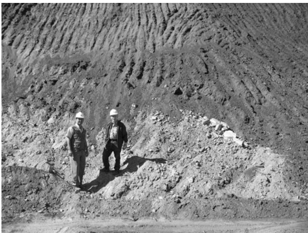
Fig. 5 Contact between hematite–talc schist ( white ) and soft hematite ore. Orlando G. Rocha Filho ( left ) and Richard D. Jones pose as scales
