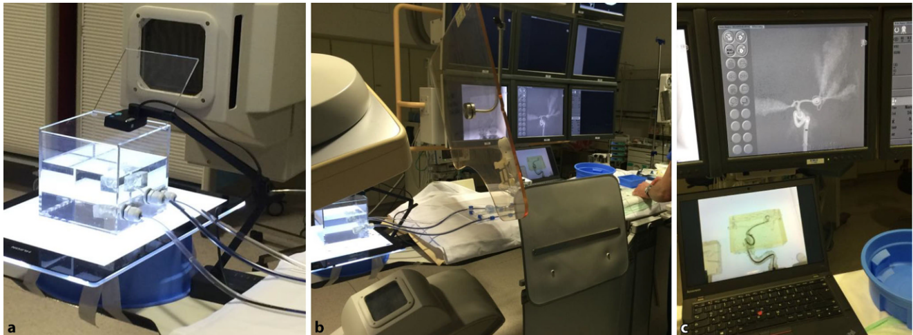
Fig. 8 ▲ Exemplary setup in the angiography suite for training of endovascular treatment of intracranial aneurysms (Flow Modella for Deployment of Devices in Aneurysms, FlowModda, www.flowmodda.com ). a The three-dimensional (3D) model is connected to a fluid circulation system and immersed in water inside the transparent box representing a patient's head. b The model is accessed through silicone tubing with standard angiographic equipment, simulating transfemoral approach. c A transparent 3D model allows for parallel imaging by angiography (upper flatscreen monitor) and USB camera (laptop screen)
