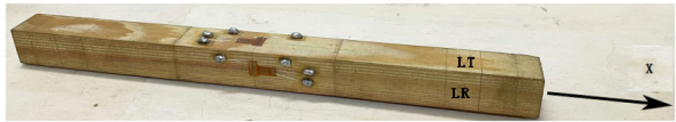
Fig. 9 Test specimen (larch) for four-point bending: Definition of fiber direction and wood grain
