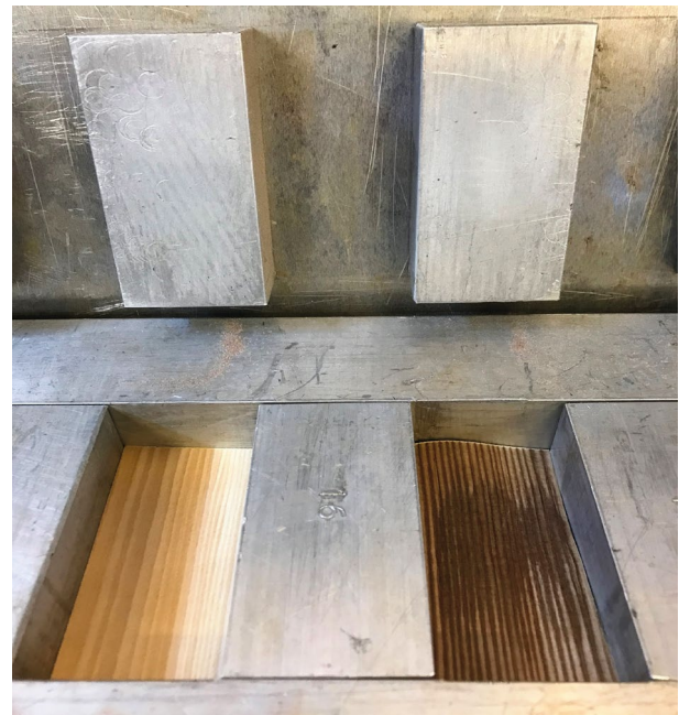
Fig. 1 Aluminum press form with native spruce veneer (left), and chemically treated and hot-pressed spruce veneer (right)
