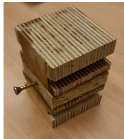
Fig. 2 IB test used to measure the tendency towards splitting for the samples: a inserting a screw into the core layer; b prepared sample for testing
