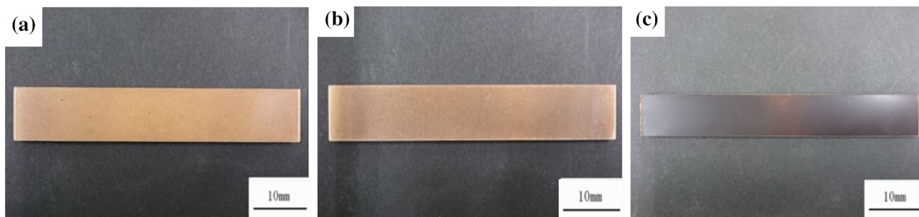
Fig. 9 Surface images of bamboo powder specimens molded at a 160 °C, b 180 °C, and c 200 °C
