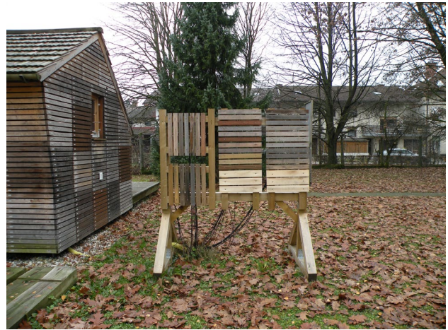
Fig. 2 Stand for the horizontally and vertically exposed samples facing north nearby to the wooden model house unit at the Department of Wood Science and Technology in Ljubljana
