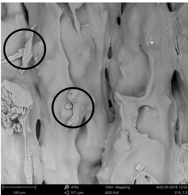
Fig. 6 This SEM picture illustrates a fracture surface of a FLM 3D printed tensile specimen having an infill orientation of 90^\circ using a wood filament with a fiber content of 15 wt. %. It can be seen that adjacent filament strands are only connected in a few spots (marked in black) with each other
