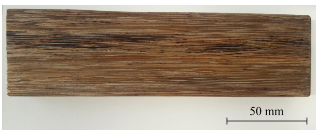
Fig. 5 Prototype of glued laminated Euterpe oleracea using the peripheral portion of the stem
