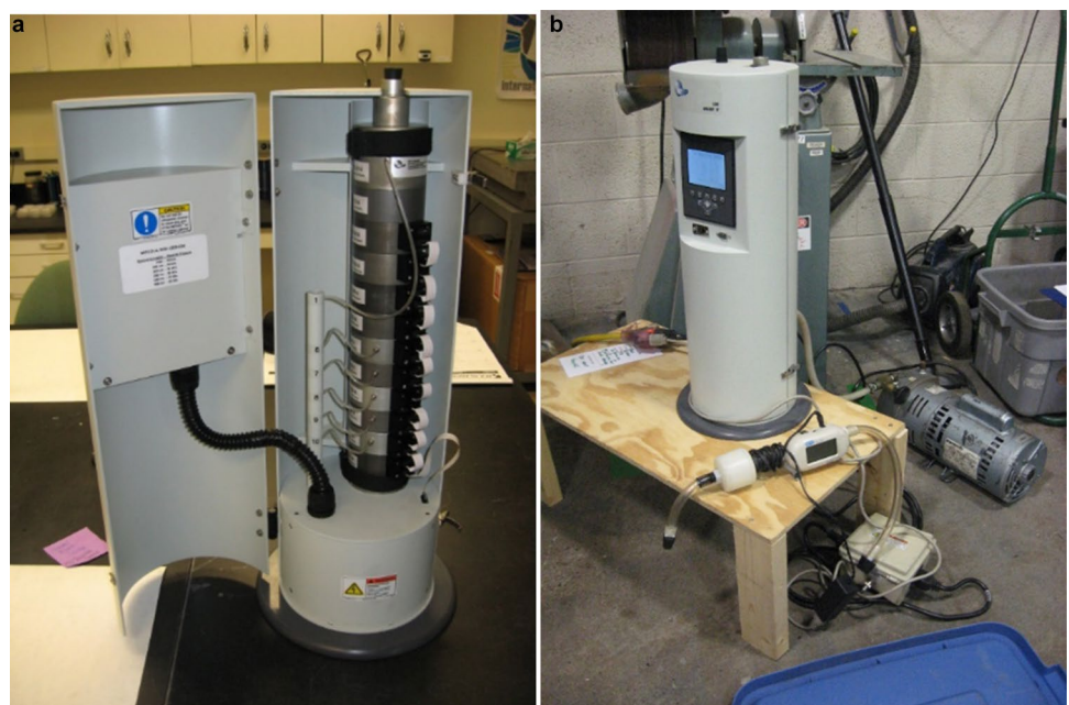
Fig. 2 a Inside the MOUDI impactor showing the individual stages. b MOUDI impactor and flowmeter test setup
